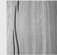
SC Soft cracks
