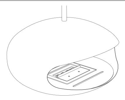
Once all spilled or residual fuel has been wiped clean, and all other forms of fuel have been sealed and moved to a safe distance from the Combustion Chamber, and the Combustion Chamber has been placed back inside the Chimenea as indicated above, it is safe to consider igniting the Combustion Chamber.
