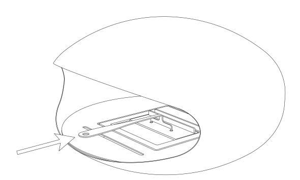
To extinguish the flame, insert the tips of the *Sliding Lid Handle* into the holes of the *Sliding Lid* of the *Combustion Chamber* and slide all the way forward until the flame is extinguished.
