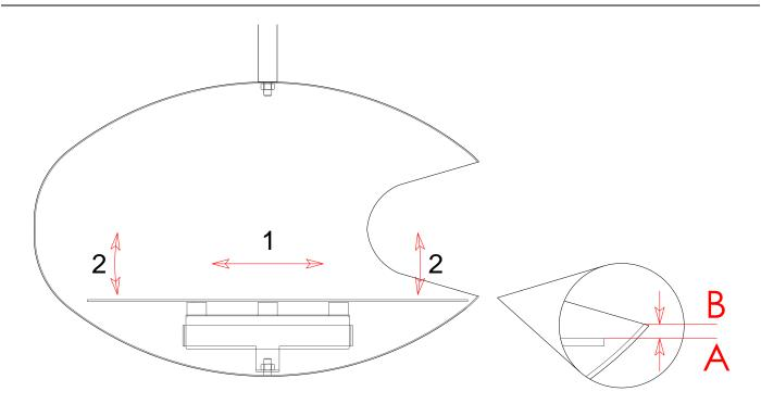
By finely adjusting the Removable Tray Bracket backward and forward (1) allows for the necessary adjustment in height (2) of the Mount Plate.
