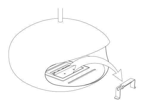
Your Cocoon Burner is now ready to use, follow the steps on the following pages to correctly and safely fill, ignite, adjust, shut off and refill the Combustion Chamber. Always make sure the Lifting Handles are removed from the Combustion Chamber as shown above when it is not in use otherwise these parts will become too hot to touch and may cause injury.
