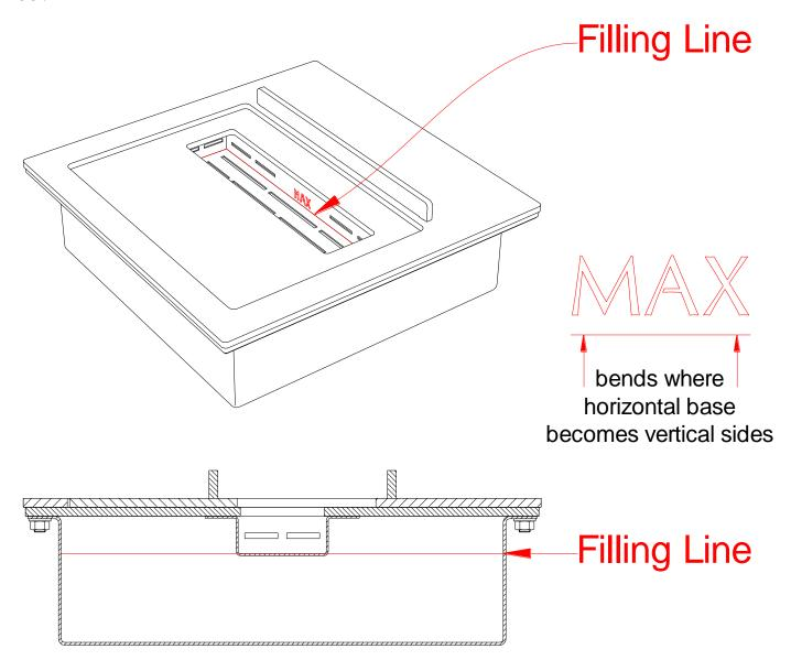
To fill the Combustion Chamber, remove it from the Main Body using the Lifting Handles and pour fuel inside the Vent Opening being careful not to spill. Fill up to the fill line as indicated in red with no more than 1.5L of fuel (3-5 hrs burning time). After filling is done, wipe away any spilled or excess fuel before returning the Combustion Chamber to the Mount Plate opening.
