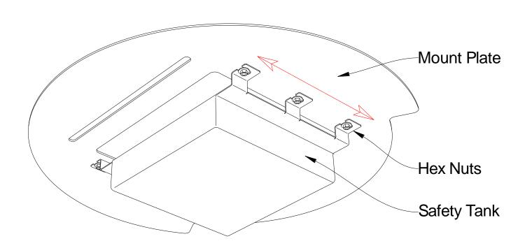
Further adjustment to the position of the Mount Plate can be achieved by loosening the 6 hex nuts below the Mount Plate and sliding the Safety Tank front to back slightly. Always make sure that the Safety Tank below the Mount plate is properly secured after this adjustment.
