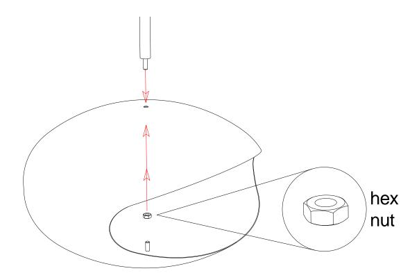
Position Main Body into hanging bar and secure from inside with wing type nut.
