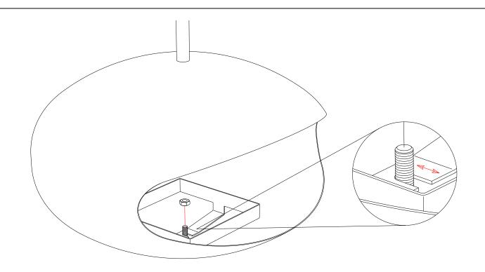
Position the Movable Tray Bracket over the threaded stud at the base of the Main Body and adjust according to the instructions on the following page before securing with hex nut.
